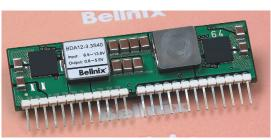
Figure 1 Designers usually dismiss point-of-load supplies as too simple to benefit from digital-control techniques, but this 40A supply from Bellnix incorporates a Volterra digital controller for less than \$30.
