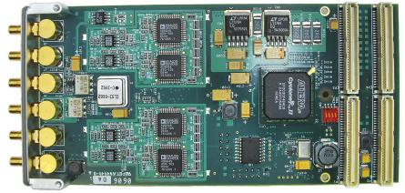
The Tetra-PMC+ board features four ADCs operating as fast as 105 MHz and a Cyclone II FPGA providing control, data distribution, and front-end processing.
